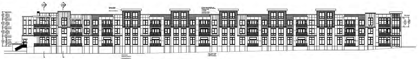
1 Building 1 Front Elevation Scale: 1/8" = 1'-0" Type: 9A Construction
